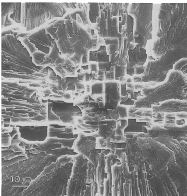
Figure 6 Scanning electron micrograph of damage zone generated by a lower absorbed energy.
